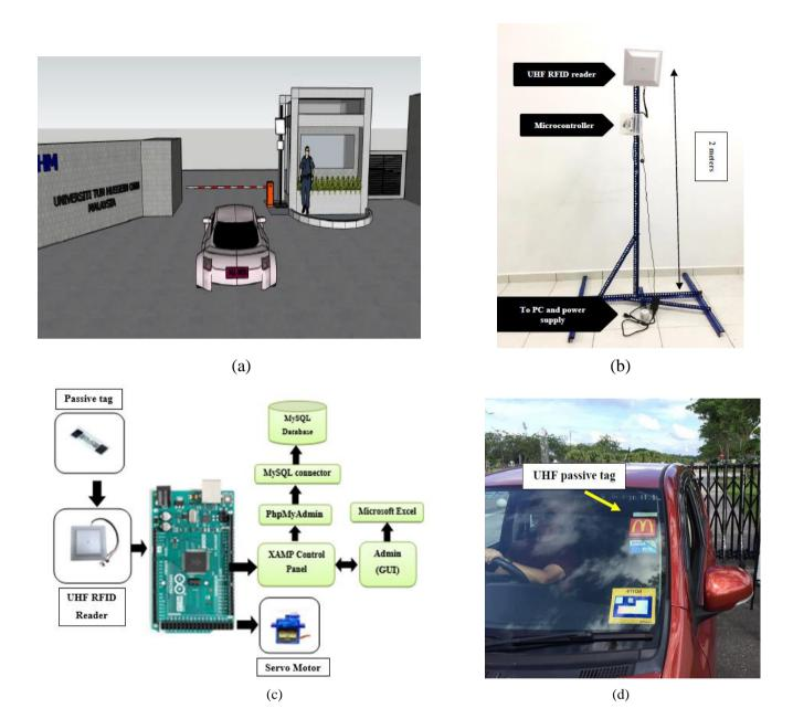
Fig. 1 - System's set up; (a) Overall system's placement; (b) Front view prototype (c) Block diagram of the system; (d) Passive tag placement.
