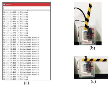
Fig 4 - (a) Serial monitor display for barrier gate status; (b) Barrier gate when tag is detected; (c) Barrier gate when no tag is detected.
