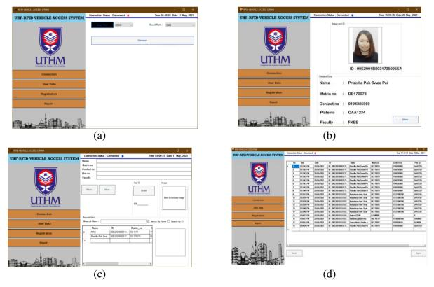
Fig. 3 - The GUI's dashboard for vehicle access system contain (a) Connection Menu; (b) User Data Menu; (c) Registration Menu; (d) Report Menu
