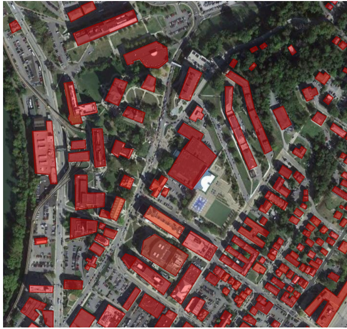
Figure 4.9: Map of WVU downtown campus. The red-highlighted buildings are the blockages, and the base stations and user are randomly placed over the region.
