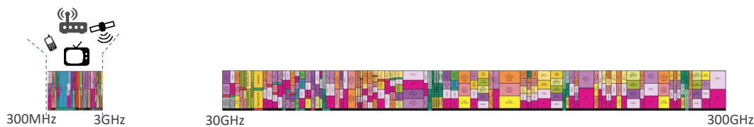
Figure 1.1: millimeter wave spectrum is the band of spectrum between 30 GHz and 300 GHz.
