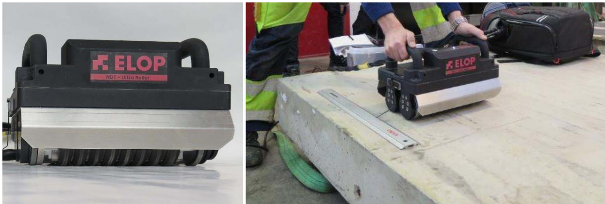
Figure 3.4: Multilayered Ultrasonic Rolling Scanner built by ELOP (Chapagain et al. 2018)
