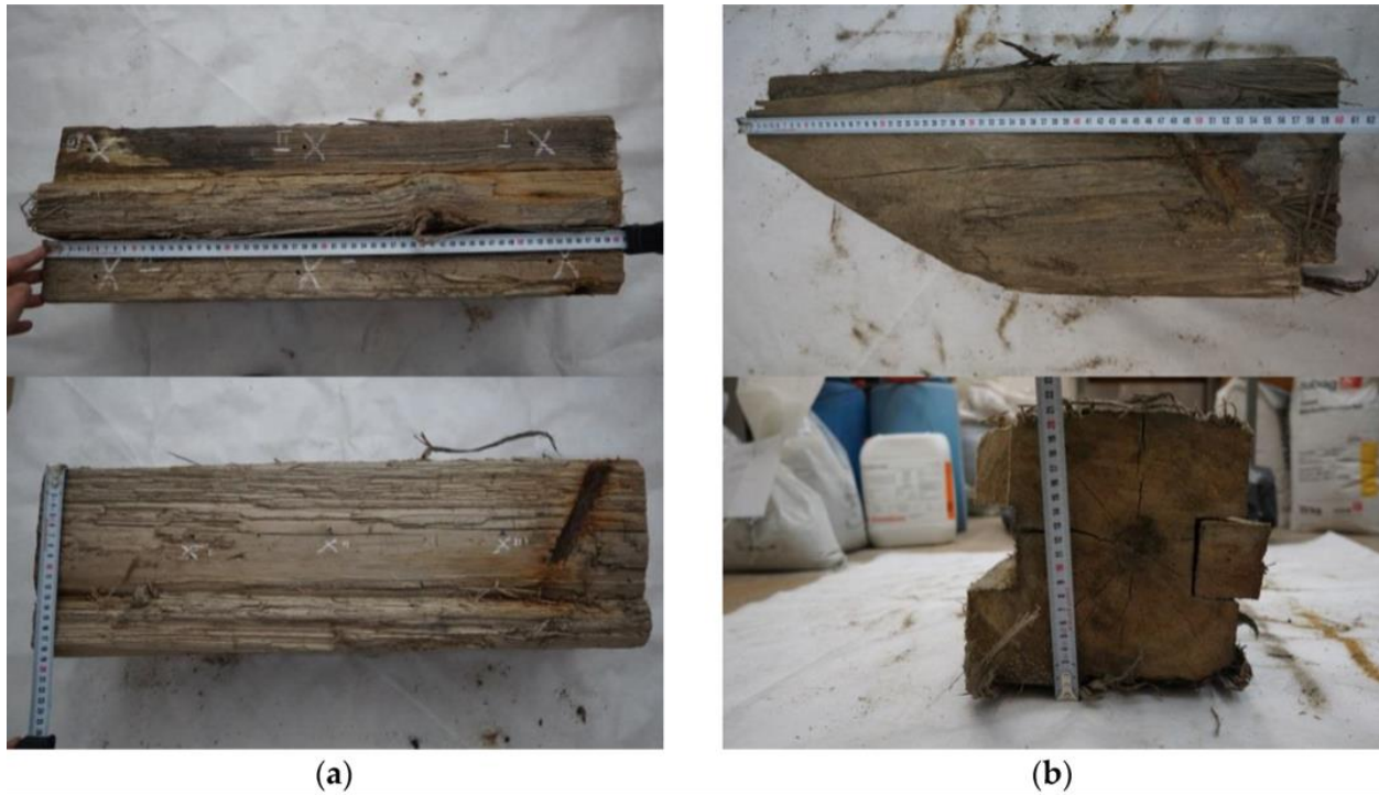
Figure 5.3: Shown are (a) sample taken for test. (b) Sample for tests with a cut (Nowak et al. 2019)
