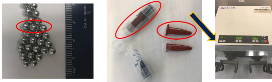
Figure 3.2: Images for the adapted homemade reaction chambers for the QuEChERS extraction.
