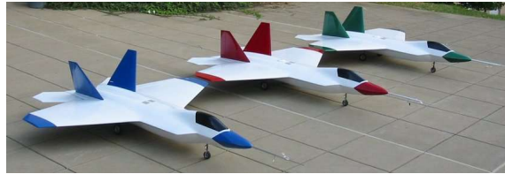
Figure I: WVU YF-22 Unmanned Research Aircraft. Photo courtesy of Dr. Marcello Napolitano.
