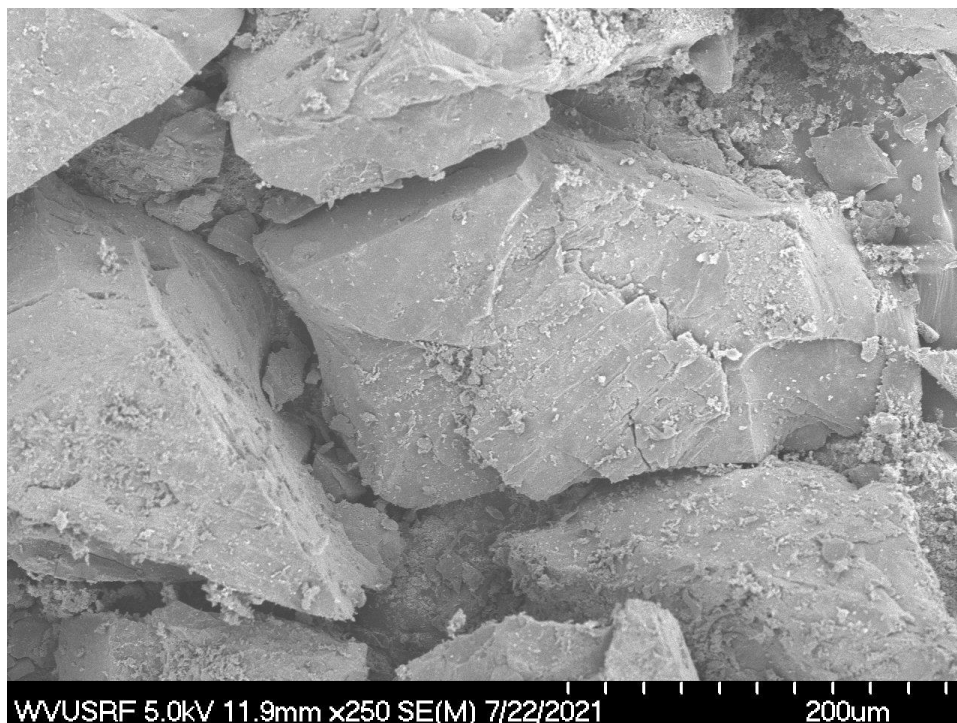
Figure 4.25: Example of PRB coal char agglomeration post MWDRM processing from \text{Fe}_3\text{O}_4 sample S4.1.4.
