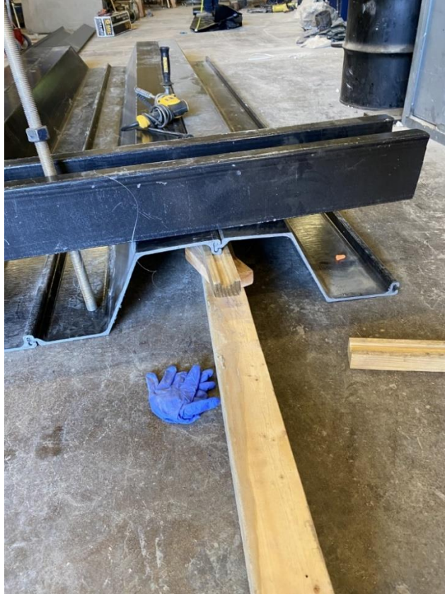
Figure 3. 5: Sheet Pile Specimen Under Construction with Wale Section
