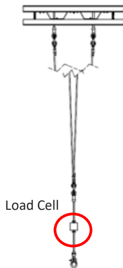
Figure 3. 12:Load Cell Location
