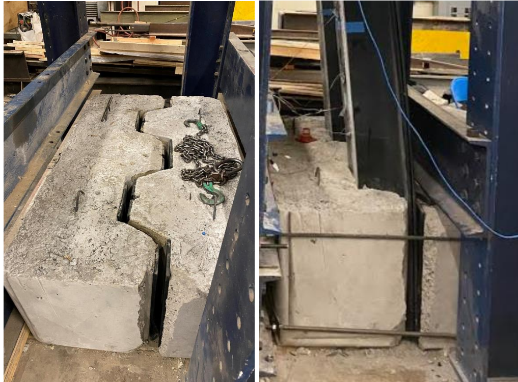
Figure 4. 12:Restraining Structure with Elastomeric Padding
