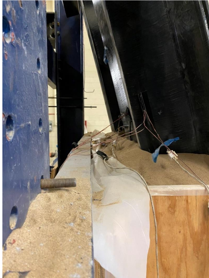
Figure 4. 2:Sheet Pile Specimen in Sand
