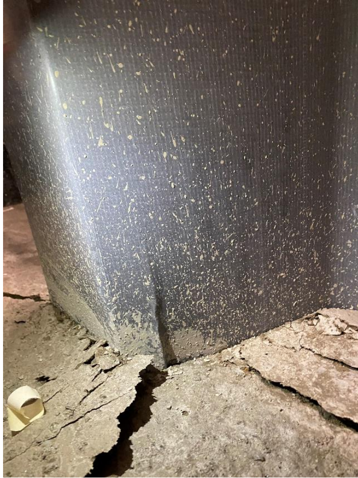
Figure 4. 34:V-Test 2 Stress Concentration
