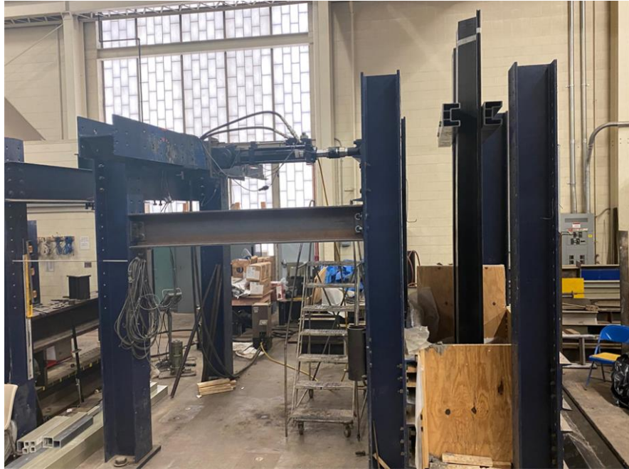
Figure 3. 3:Sheet Pile Test Specimen in Fixture
