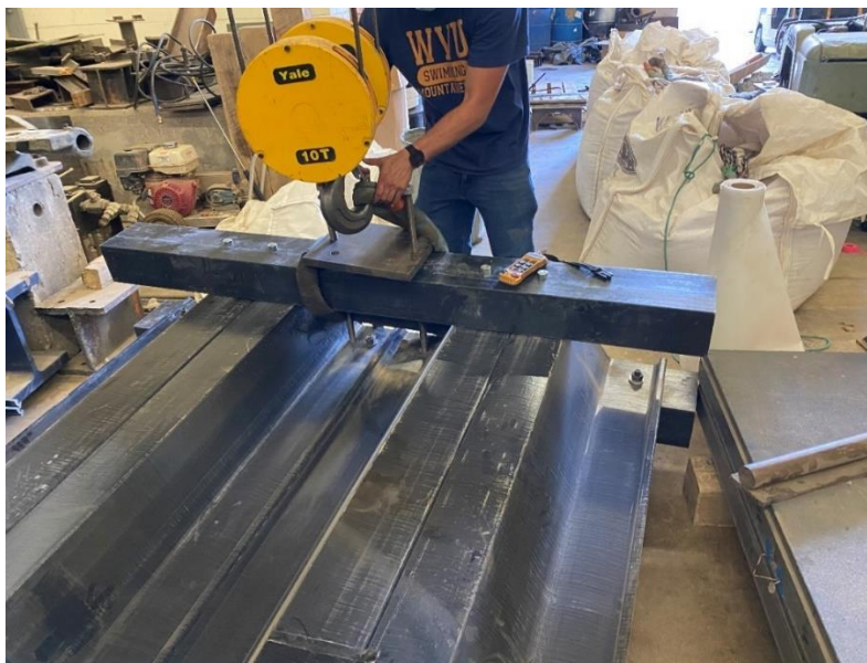
Figure 3. 4: Single Sheet Pile Specimen
