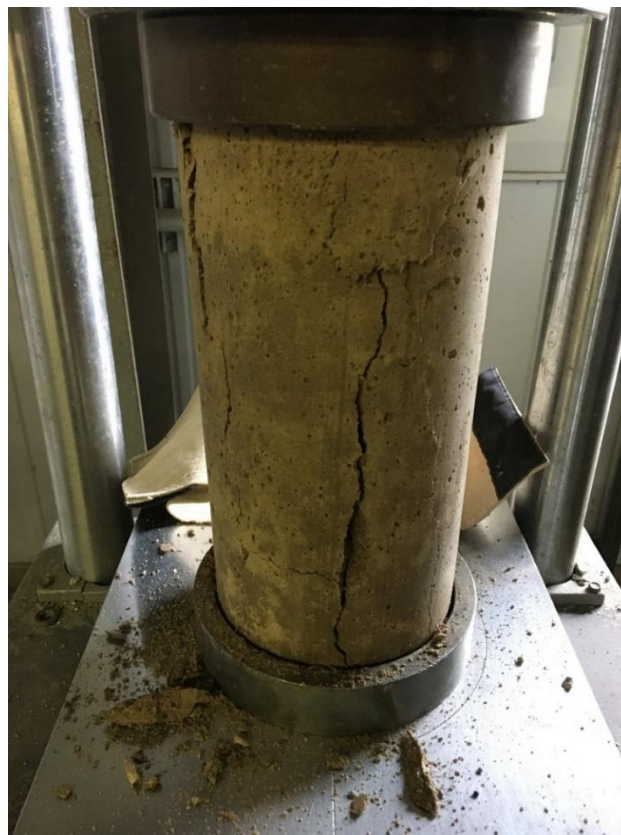
Figure 5. 17:Embedment Material Compression Test
