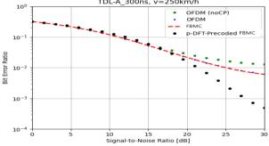
Fig. 13. BER vs SNR for 1024 Subcarriers
