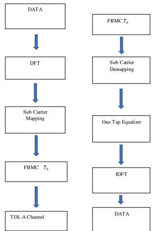
Fig.5. Block diagram of Pruned DFT Precoded FBMC
