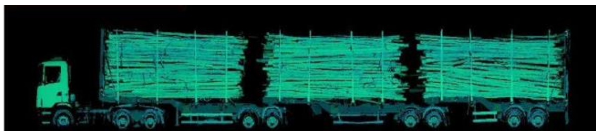
Figure 1. 3D image generated by road train's Logmeter® 4000.
