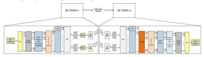
Fig. 1. DCO-SC-FDM for underwater communication systems using duo lasers.
