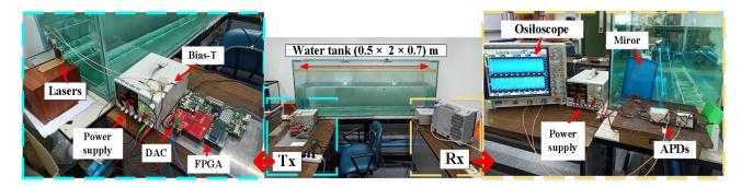
Fig. 2. Experimental setup of UOWC SC-FDM communication systems.
