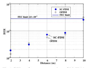
Fig. 3. BER performance comparison of SC-FDM and OFDM for 8-QAM.
