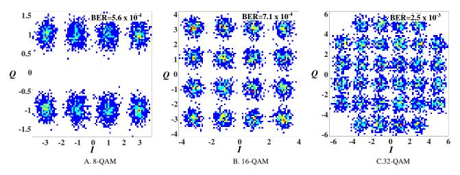
Fig. 4. Constellation plot at 6 m for: A. 8-QAM, B. 16-QAM, and C. 32-QAM for SC-FDM.
