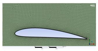
Fig. 6. Meshing Setup Close-up.
