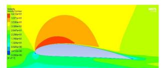
Fig. 11. Velocity Contours at AoA = 4 & H/C = 0.1.
