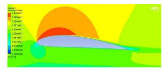
Fig. 15. Velocity Contours at AoA = 4 & H/C = 0.2.
