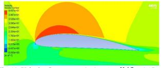
Fig. 13. Velocity Contours at AoA = 4 & H/C = 0.15.
