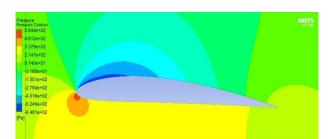
Fig. 12. Pressure Contours at AoA = 4 & H/C = 0.15.
