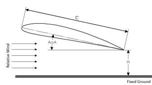
Fig. 1. Definition of AoA and Ground clearance.
