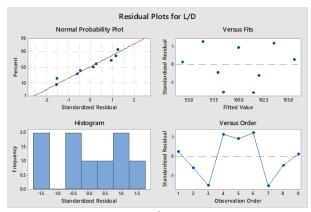
Fig. 20. Residual plots for L/D deviation of the fitted regression.
