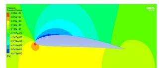
Fig. 14. Pressure Contours at AoA = 4 & H/C = 0.2.
