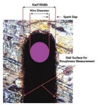
Figure 2: Measurement of kerf width and surface roughness
