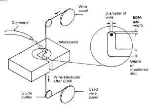
Figure 1: Basic feature of WEDM sets up
