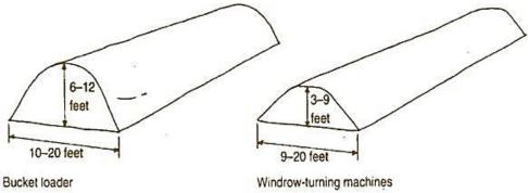
*Figure 11. Typical windrow shapes and dimensions, (Source:* https://content.ces.ncsu.edu/large-scale-organic-materials-composting)
