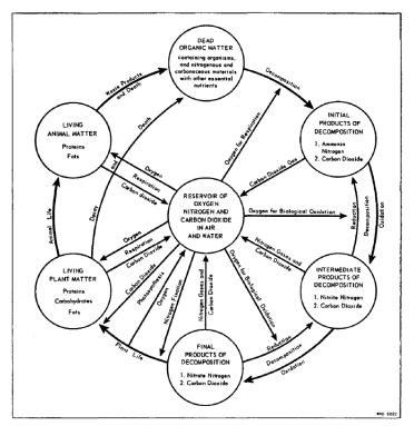
Figure 3. Cycle of nitrogen and carbon in aerobic decomposition, (Harold B. Gotaas, 1956)
