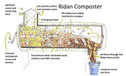
Figure 9. Ridan Composter, (Source: http://www.ecovrs.com/en/products/in-vesselcomposting/ridan-composter/)
