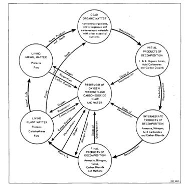
Figure 4. Cycle of nitrogen and carbon in anaerobic decomposition, (Harold B. Gotaas, 1956)
