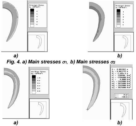
Fig. 5. a) von Mises equivalent stresses, b) The set of results for the point in the Figure
