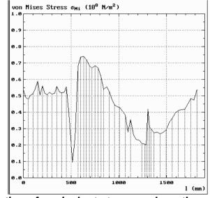
Fig. 7. Variation of equivalent stresses along the entire contour of the stilt
