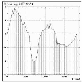
Fig. 8. Variation of tangential stresses  $\tau_{XY}$  on the entire contour of the stilt
