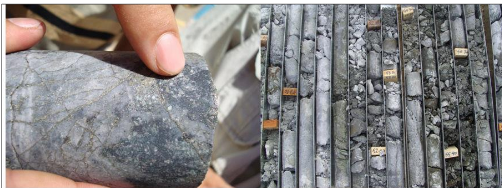
Figure 2. A View of Drilling Cores As Well As Calopyrite Mineralization Can Be Seen in One Core. Source: Authors (2020).
