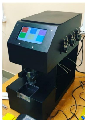
Gambar 3. Smart bartender with peristaltic pumps
