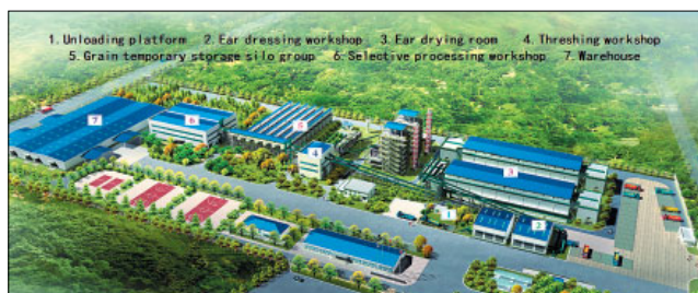
Fig. 7. Layout of large-scale corn seed processing plant
