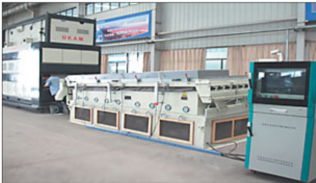
Fig. 3. Hydraulic gravity separation test detection platform
