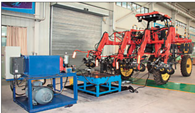
Fig. 4. Hydraulic testing platform
