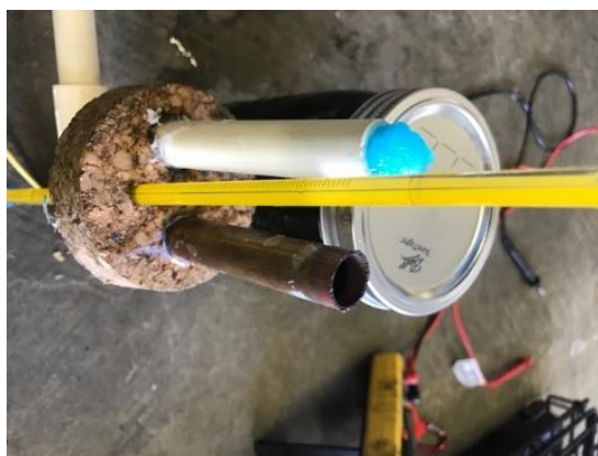
d) The “standard” copper – copper (II) sulfate cell. Copper pipe (pure) was used as the cathode. A laboratory thermometer ensured the temperature was near 25° C when the measurements were taken.
