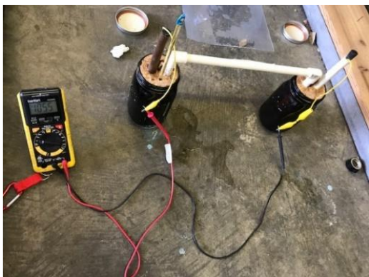
a) Entire Apparatus: Half – Cells (Jars) and Salt Bridge with 1M KCl Solution.
