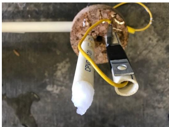
c) The Zinc anode consisted of a zinc – plated bracket connected as shown. It proved suitable and gave a decent measurement of the reduction potential of zinc.
