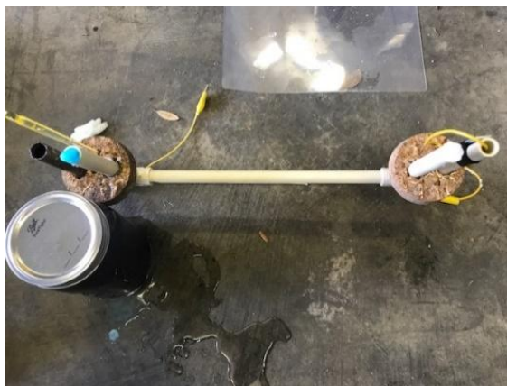
b) Salt – Bridge and electrodes as taken from service in testing the chemistry. Cotton in the salt bridge tubes slows diffusion inside it.
