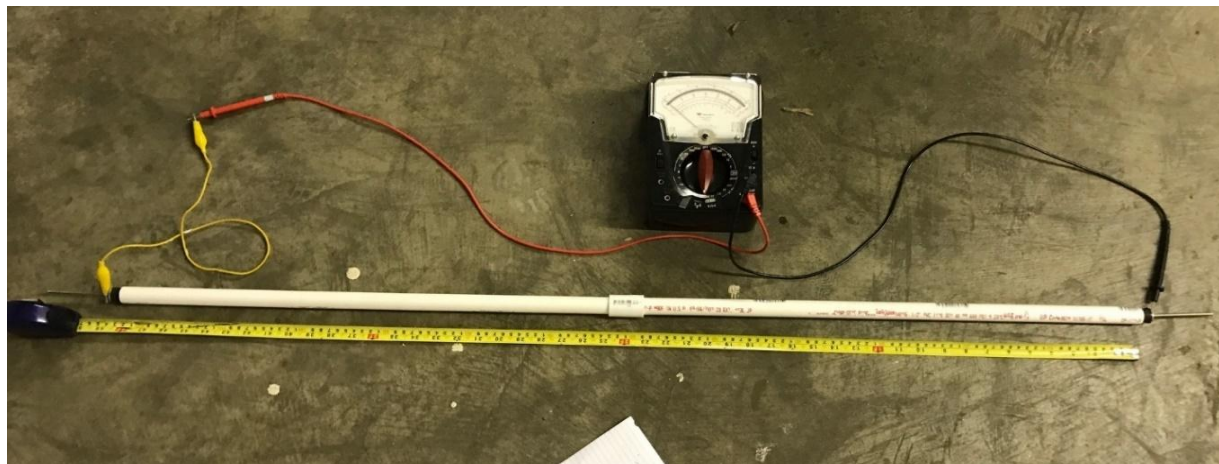
Figure 10. Experimental apparatus for the above ionic conductivity experiment. The pipe contained 0.1 M / L potassium chloride, in distilled water. The meter measured the resistance.
