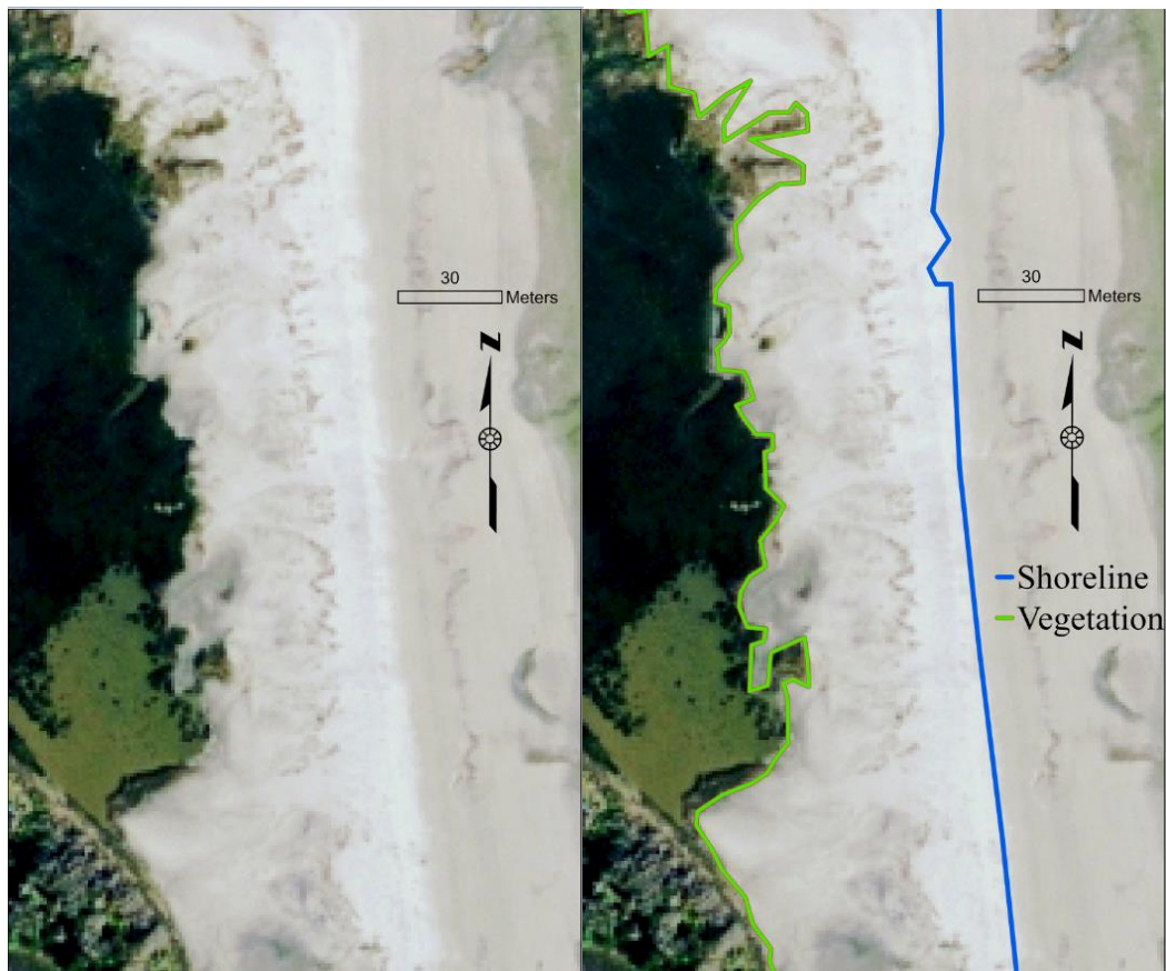
Figure 3-4: Digitization example. 2013 imagery at a 1:1000 scale from the southern section before and after the vegetation and shoreline were manually digitized.
