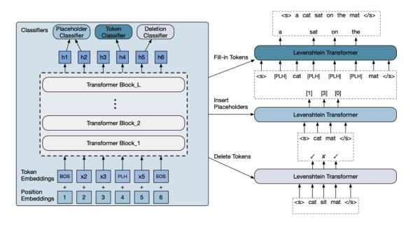
FIGURE 2.5: The structure of levenshtein Transformer network.
