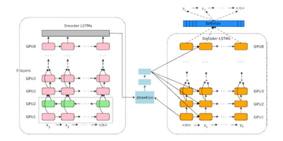
FIGURE 2.2: The structure of GNMT model. The first two layers in the encoder are forward and backward LSTM layers.
