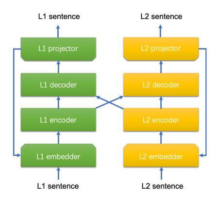
FIGURE 2.6: The structure of unsupervised neural machine translation models.
