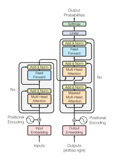
FIGURE 2.3: The structure of Transformer network.
