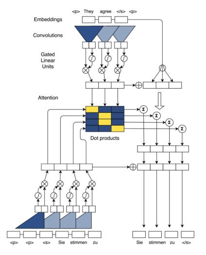
FIGURE 2.4: The structure of convolutional NMT network.
