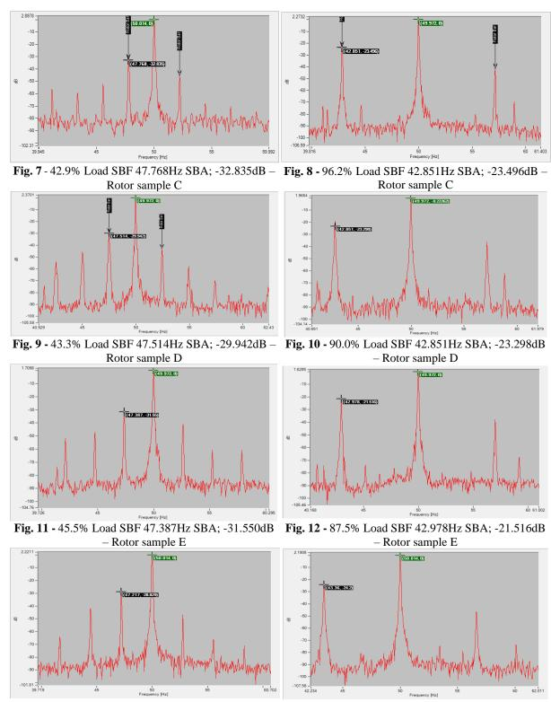
Fig. 13 - 56.1% Load SBF 47.217Hz SBA; -28.829dB Fig. 14 - 102.5% Load SBF 43.360Hz SBA; -24.200dB Rotor sample F – Rotor sample F
