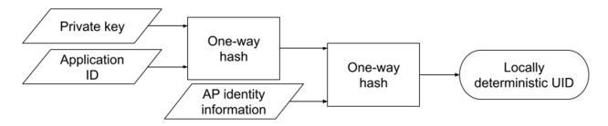
Fig. 1. Flowchart detailing the generation of a locally deterministic UID.
