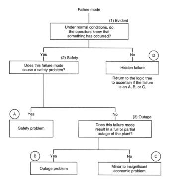
Figure 2. Logic Tree Analysis Diagram
