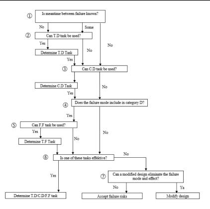
Figure 3. Selection Action Diagram
