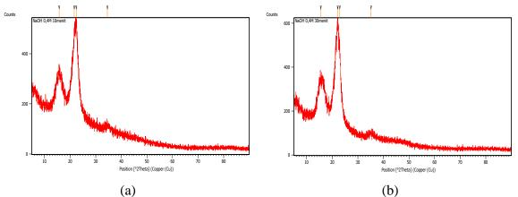
Figure 4. XRD Pattern of Sugarcane Bagasse for (a) 10 minutes and (b) 30 minutes
