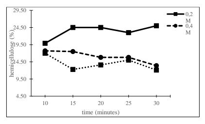
Figure 3. The Effect of Reaction Time and solvent Concentration on the Percentage of Hemicellulose
