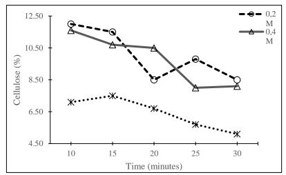
Figure 2. The effect of Reaction Time and Solvent Concentration on the Percentage of Cellulose
