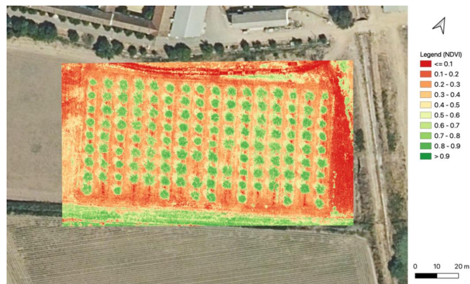
Figure 2. NDVI orthomosaic of the experimental orchard printed on PNOA RGB orthomosaic ( https://pnoa.ign.es , accessed on 6 April 2021). Day of year 216.
