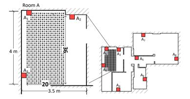
Fig. 1 The map of the experimental environment with the red boxes denote anchor nodes
