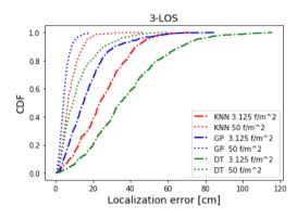
Fig. 2 CDF of the localization errors of ML algorithms for 3-LOS case and fingerprint densities of  $50 f / m^2$  and  $3.125 f / m^2$
