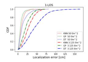
Fig. 4 CDF of the localization errors of ML algorithms for 1-LOS case and fingerprint densities of  $50 f / m^2$  and  $3.125 f / m^2$
