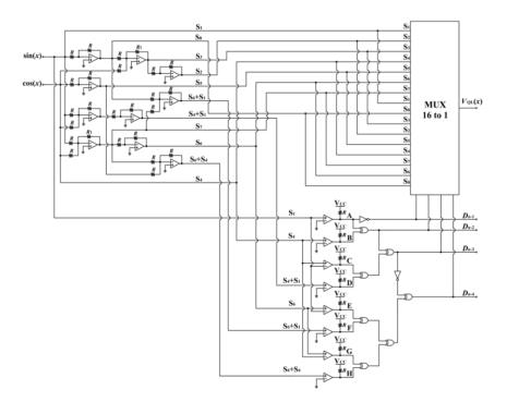
Fig. 1 A 4-bit mixed analog-digital circuit
