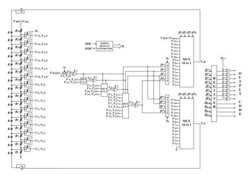
Fig. 3 An 8-bit two-stage nonlinear ADC of a compact design
