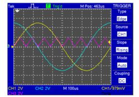
Fig. 5 Sine (CH1), cosine (CH2) and quasi-linear signal (CH3) displayed using Tektronix oscilloscope
