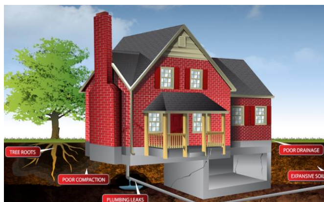
Fig. 2 Causes of damage of foundations and superstructure [1]
