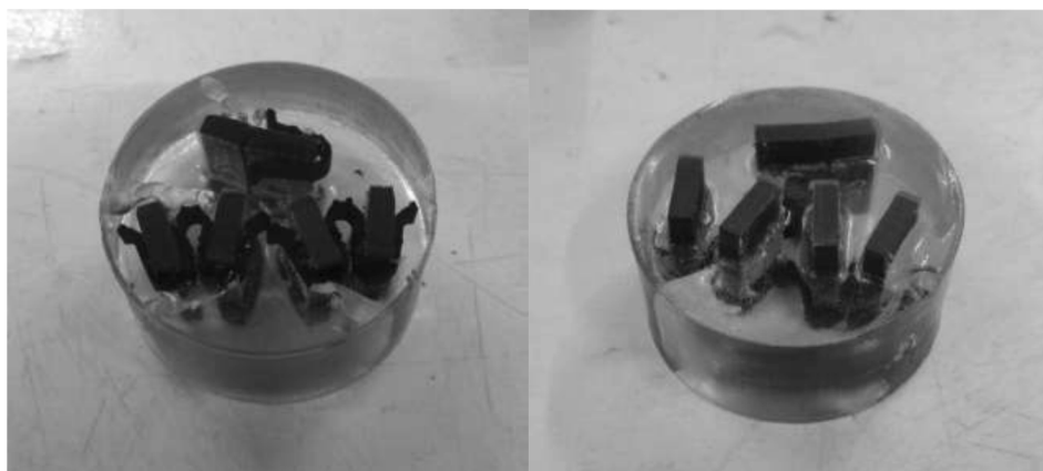
Fig. 9. potted 3D printed polymer composites specimen for micro sectioning.
