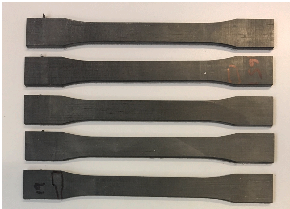
Fig. 4. Dog bone shaped tensile samples extracted from large plate using water jet machine.
