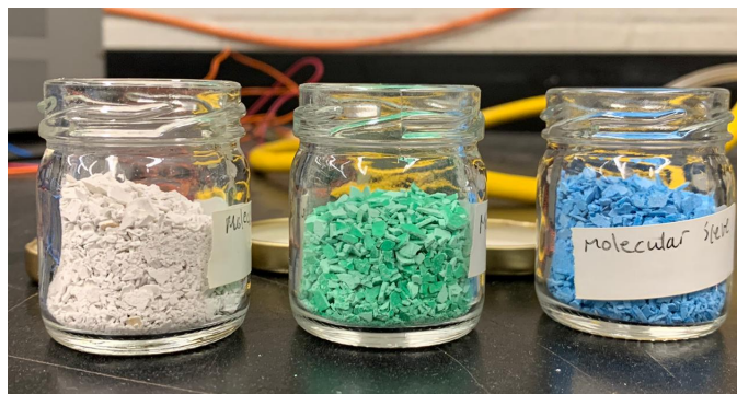
Figure 2.4. Photographs of the (a) white, green, and blue molecular sieve (MS) desiccants, and the (b) silica gel desiccant.
