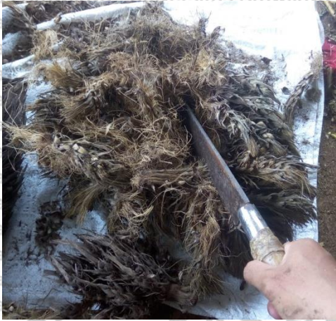
The Process of Chopping the OPEFB and Banana Stems
