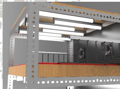
Gambar 4.2 Peletakan Lampu LED T5 6 watt
