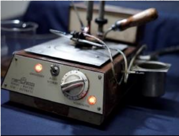
Gambar 3.4 Flash Point Tester
