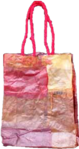
Bag made of sheets produced from fermentation of brewed tea, pulp of fruit juice and coconut water.
