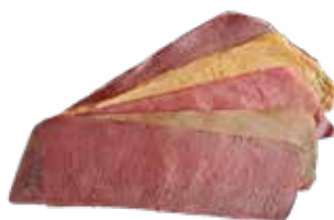
Leather-like sheets made from fermentation of brewed tea, pulp of fruit juice and coconut water.
