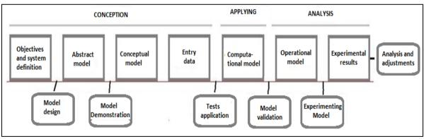
Figure 1: Simulation process in blocks Source: Adapted from De Freitas Filho (2008)
