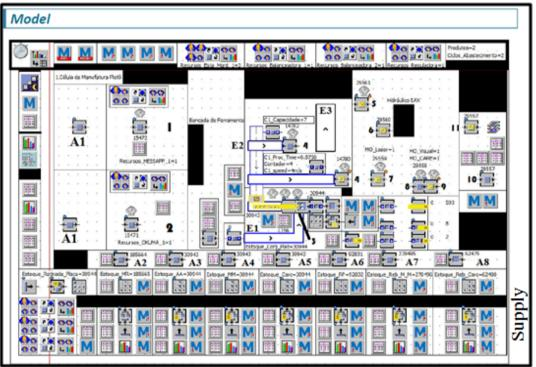
Figure 2: Layout of each Manufacturing Cell. Source: Authors (2020).
