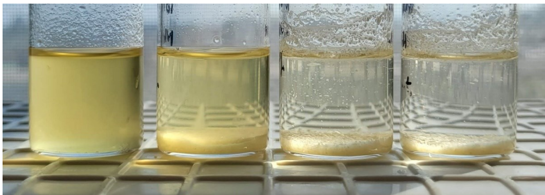
Figure 4.25: Solubility of OPF-NSblc in different bases. From left: 10% NaOH, 10% aqueous ammonia ( \text{NH}_3 ), 10% urea, 1% tetrabutylammonium chloride.
