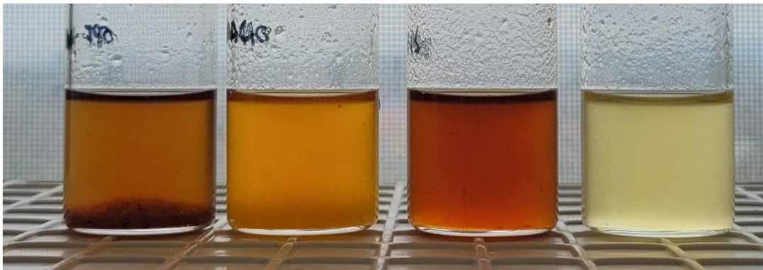
Figure 4.15: OPF biomass in 10wt% NaOH solution. From left: Raw OPF, OPF-NAAC, OPF-NS, OPF-NSblc
