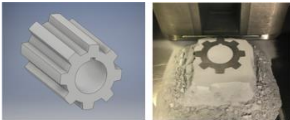
Figure 7-2: CAD design and 3D printed prototype inside the build chamber
