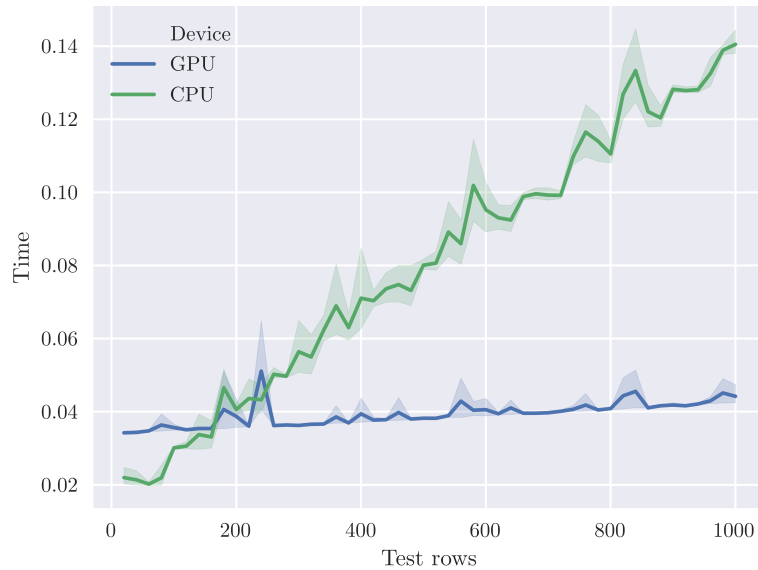
Figure 4. The crossover point where the V100 GPU outperforms 40 CPU cores occurs at around 200 test rows for the cal_housing-med model.
