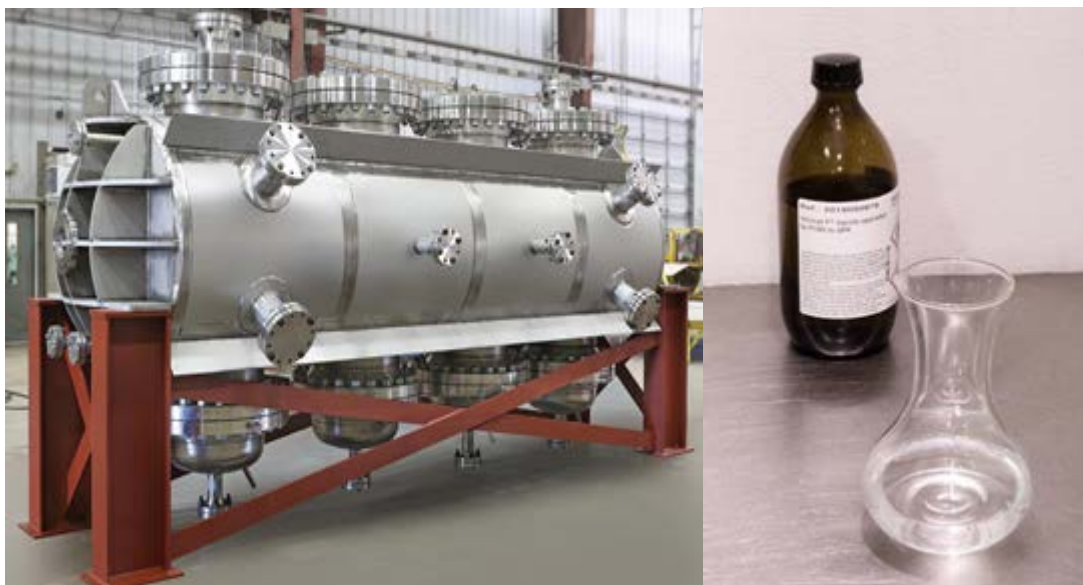
Figure 12. Velocys Fischer Tropsch reactor (above) and the finished product, SPK (right)
