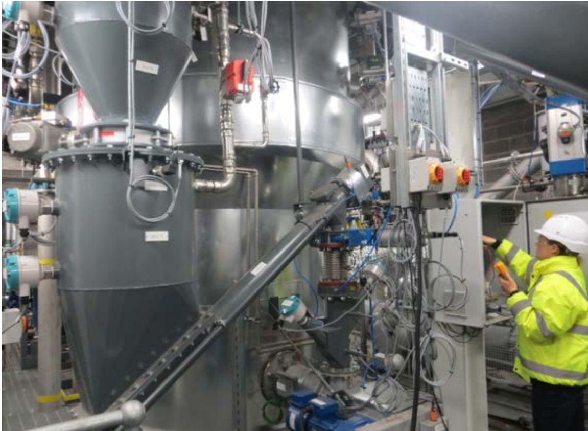
Figure 4. 1MW fluidised bed gasifier at the Energy & Bioproducts Research Institute (EBRI), Aston University.
