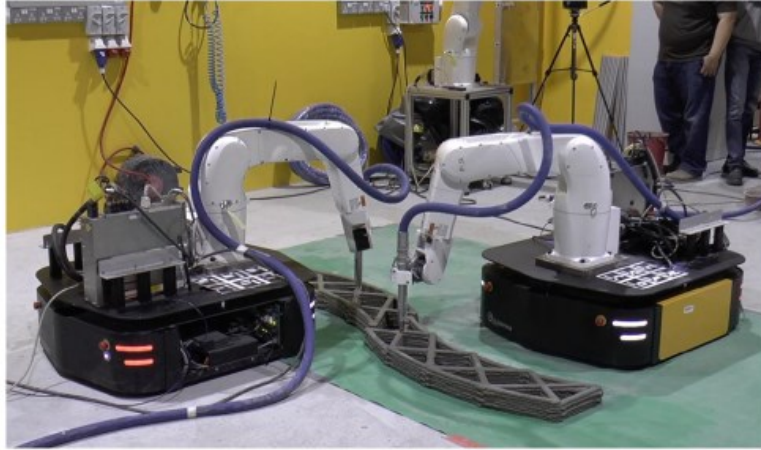
Figure 16 Twelve-DOF AM system developed in (Zhang et al. 2018).
