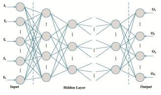
Fig. 1 — Structure of DNN
