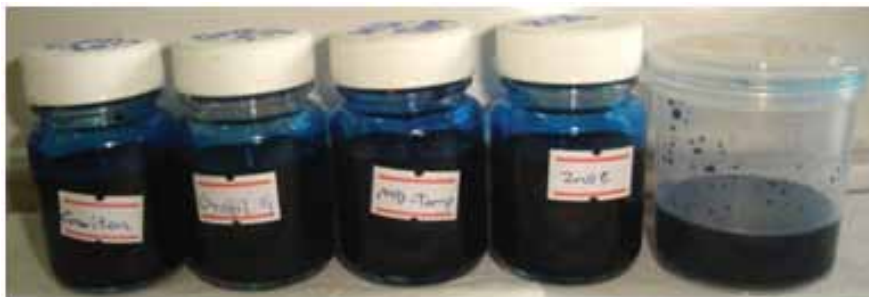
Fig.6.Specimens immersed in dye solution
