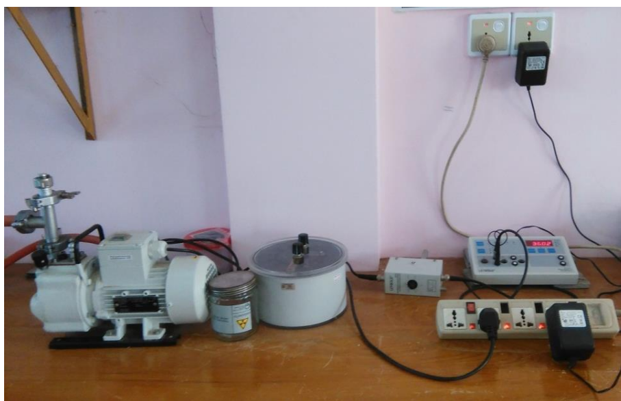
Figure 2. Alpha scattering experimental set up in Physics Department, Monywa University of Research Centre
