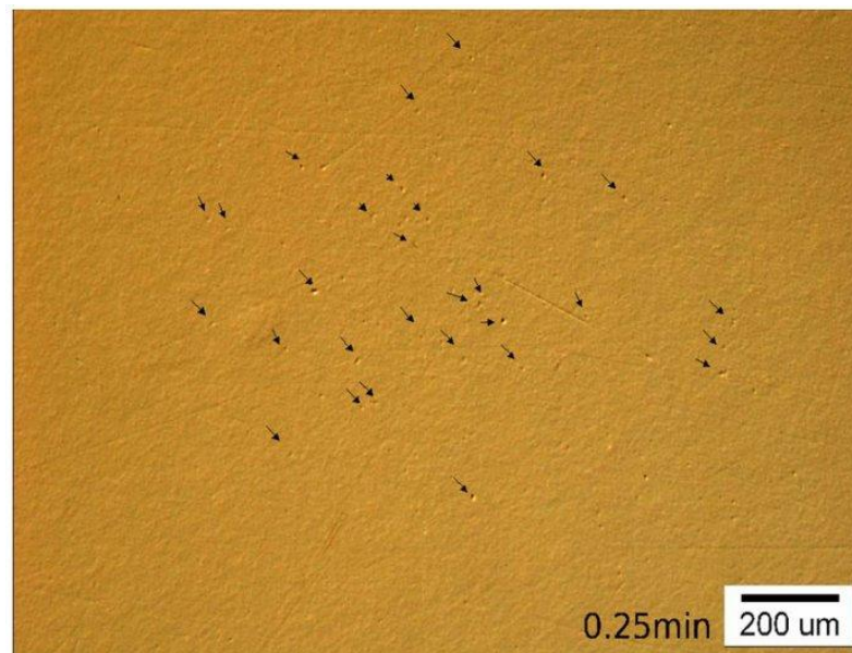
Figure 4.1 Pseudoplastic deformation pits in silicon nitride “A” that have been produced in 15 seconds of cavitation exposure. (Optical microscope).
