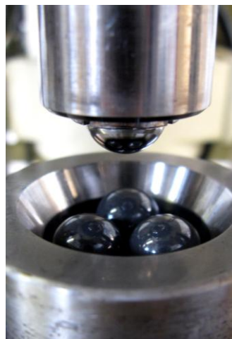
Figure 2.3 Rolling contact set up.
