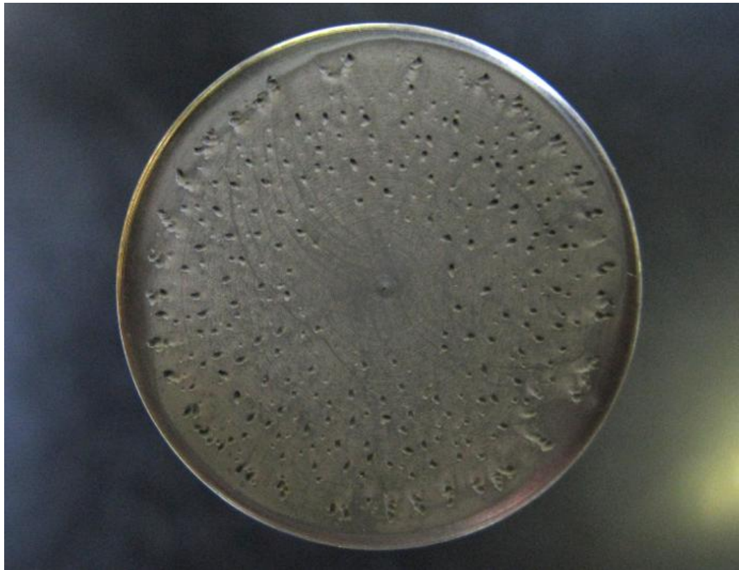
Figure 5.12. Repetitive pattern of cavitation erosion in an ultrasonic horn of 20 mm diameter.
