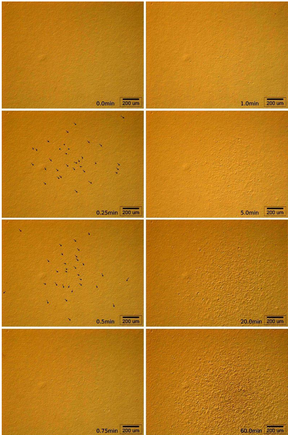
Cavitation erosion of silicon nitride "A". Time of exposure indicated.
