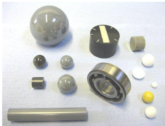
Figure 1.2 Silicon nitrides (balls and rods), alumina (specimen) and zirconias (rod and balls).
