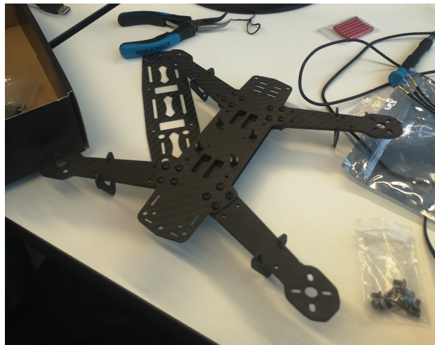
Figure 17: complete Drone Frame assembly
