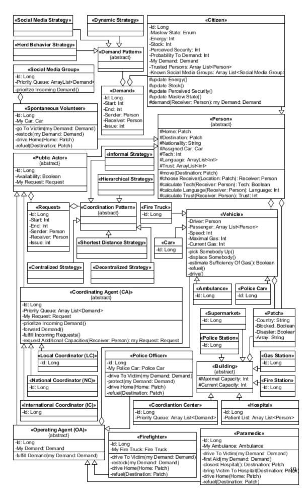
Figure 3.2: Class Diagram of the Agent-Based Model
