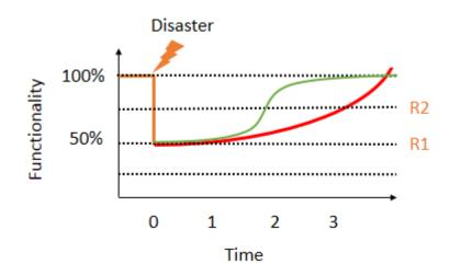
Figure 2.4: Recovery Curves According to Platt et al. (2016)
