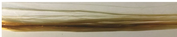
Fig. 4.4.2: First result of microwave heated PAN fiber.
