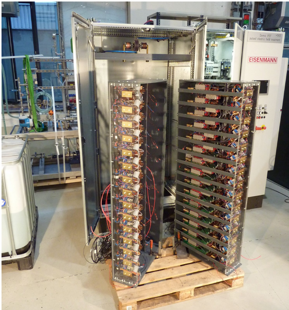
Fig. 2.1.2: PEF-Demo-Facility for bacterial inactivation of electrocoating process media. The facility consists of a 30 stage modular semiconductor-switched pulse generator, front, a control cabinet, middle, and the media transport unit in the rear.
