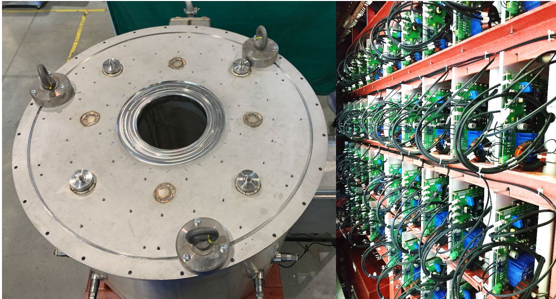
Fig. 1.8.2: Top plate of the 10.5 T magnet and electronic modules of the body power supply.
