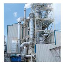
Figure 1.1: One-Effect FFE with MVR to concentrate wheat starch effluent
