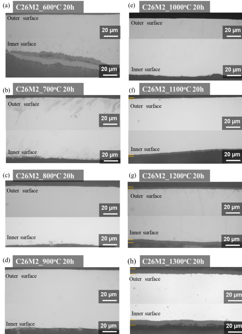
Fig 7. Optical micrographs of C26M2 after the isothermal oxidation tests at (a) 600°C to (h) 1300°C
