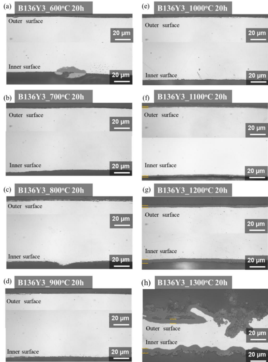
Fig 6. Optical micrographs of B136Y3 after the isothermal oxidation tests at (a) 600°C to (h) 1300°C
